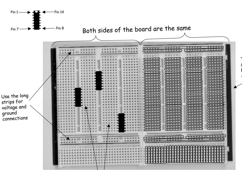
The rectangles indicate which holes are connected
